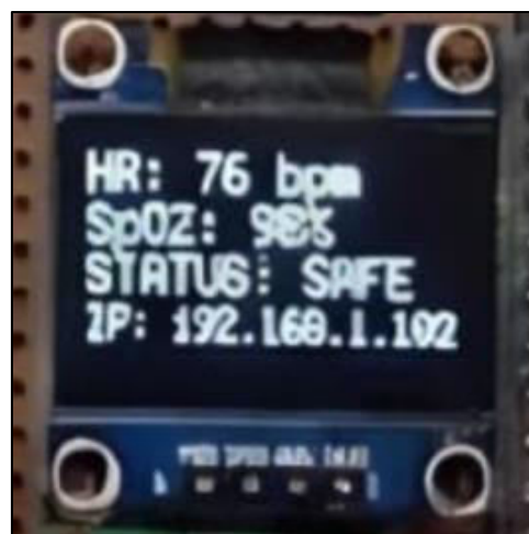
FIGURE.4. OLED DISPLAY SHOWING MEASURED PARAMETERS OUTPUT
